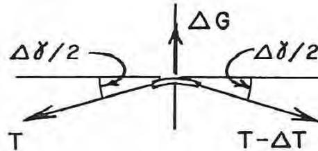
The force  $\Delta G$  is perpendicular to the segment of the loop, but may not be perpendicular to the surface of the cylinder. To find its direction, we need more solid geometry. Let's flatten out a little rectangular piece of the cylinder, of width  $R\Delta\theta$  and just high enough to contain the little piece of the sling loop.
