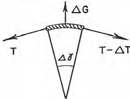
We have seen how  $\Delta\gamma$  is related to  $\Delta\theta$  and  $\Delta\phi$ . For the small angle  $\Delta\gamma$ , we may calculate  $\Delta G$  easily from the force diagram. Since  $\Delta T$  is very small,
