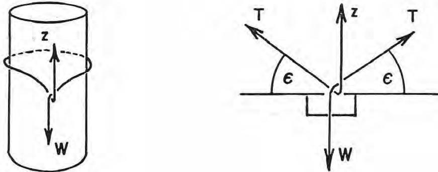
In equilibrium at the junction, the horizontal components of the tensions are equal and opposite. The vertical components will balance, too, when
