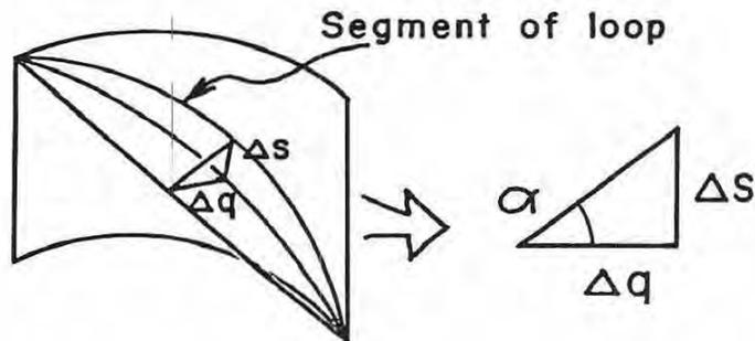
We get a little right triangle as indicated, when we draw a new straight line connecting the corners of the bent rectangle. This new line lies in the true plane of curvature of the short piece of loop. And more important, the angle  $\alpha$  is just the angle between this plane of curvature and the local perpendicular to the cylindrical surface. We see that
