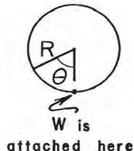
We have to use some kind of coordinate system. Looking down on the cylinder, the angle  $\theta$  designates a direction out from the center. We may let  $\theta$  be zero at the point where the weight  $W$  is supported, and it will then equal  $\pi$  radians (or  $180^\circ$ ) around back at the most distant point. By stating a value for  $\theta$ , we refer to a particular point on the loop.
